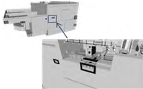
9) Detail of exit to debris recovery building. 4 channels: 1 x coarse and 1 fine filtration feed from both drum screens and one band screen; and 1 x coarse and 1 x fine filtration feed from the remaining band screen.
