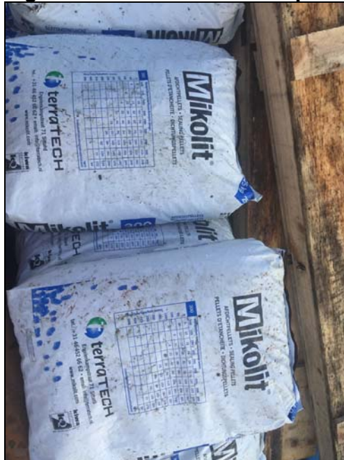
Figure 5: View of bentonite pellets used for sealing works
