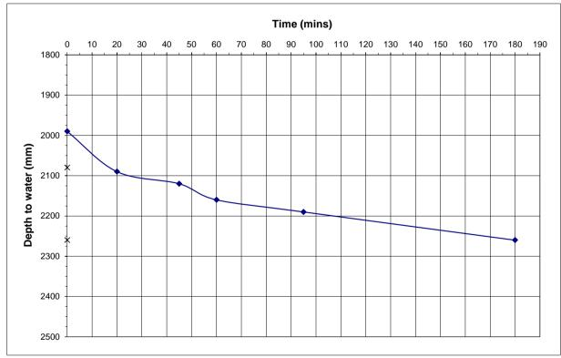
Soil infiltration rate, f, (m/s) = 9.81E-06 (Normal Test)
