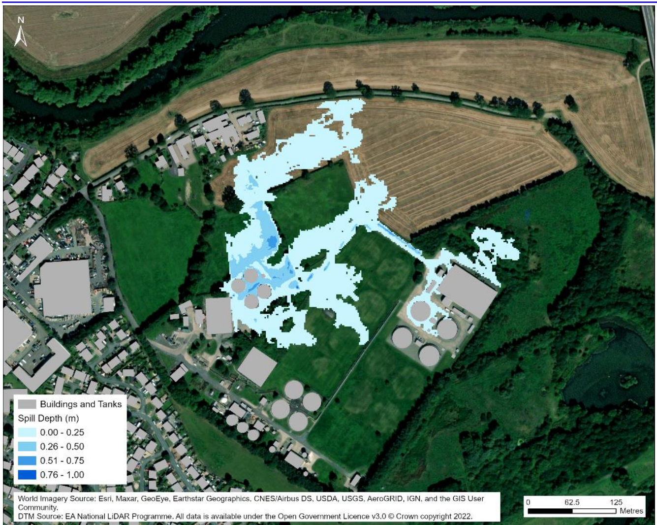
Figure 2.3 Uncontrolled spill of Monkmoor Sewage Treatment Works
