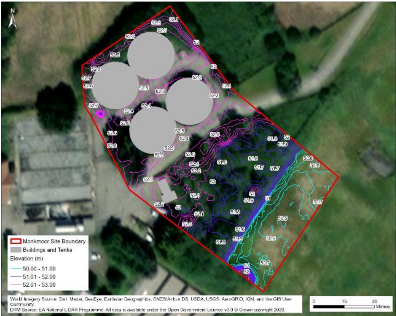
Figure 2.2 – DTM of the PKTs showing contours at 10cm intervals
