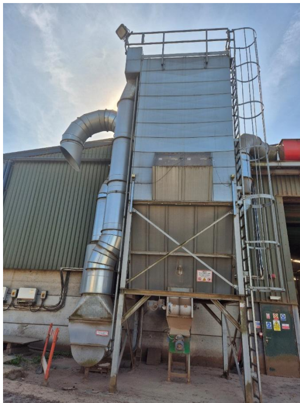
Photo 6: New permitted area – Wood milling building with dust abatement (ID 3 on Site Layout Plan))
