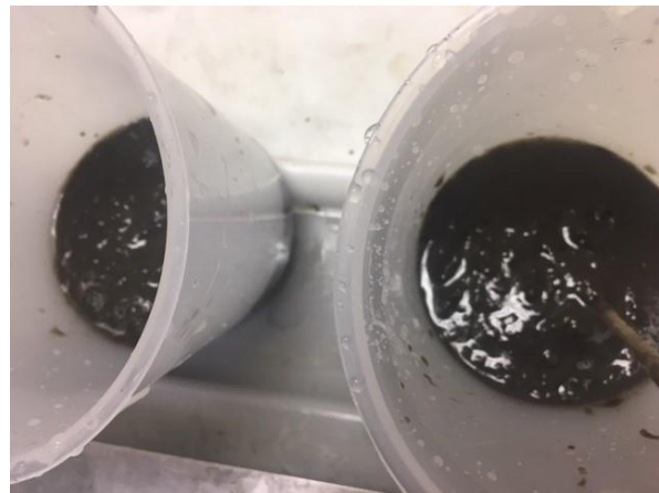
Figure 3: 4% DS sludge looks significantly thicker
