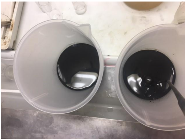
Figure 2: 2% DS sewage sludge is watery
