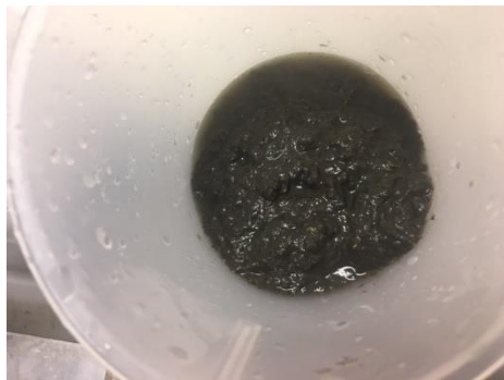
Figure 2: 2% DS sewage sludge is watery
