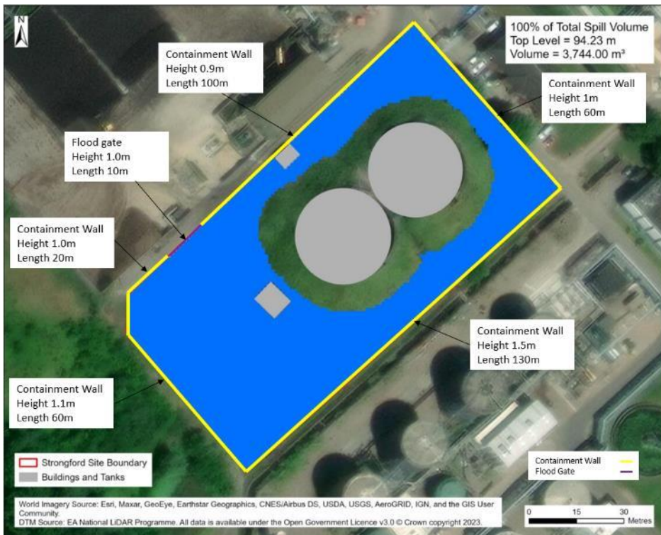
Figure iii – recommended solution for the sludge storage tank area
