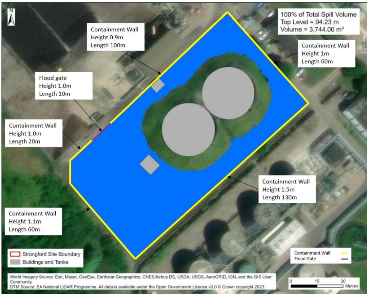
Figure 3.5 - Recommended modifications to provide secondary containment
