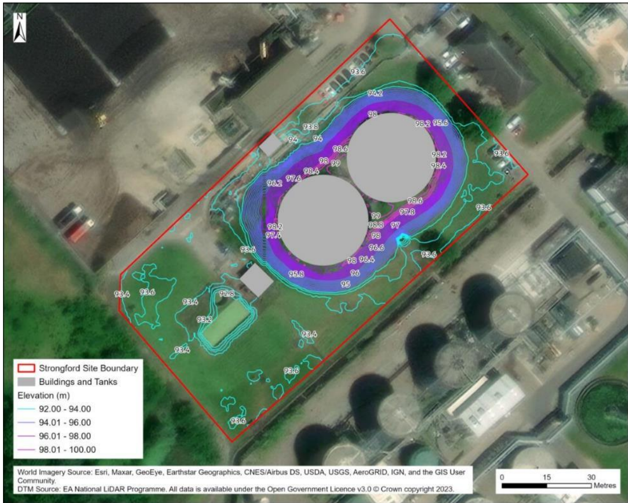
Figure 3.2 - DTM of the sludge storage tank area showing contours at 10cm intervals.
