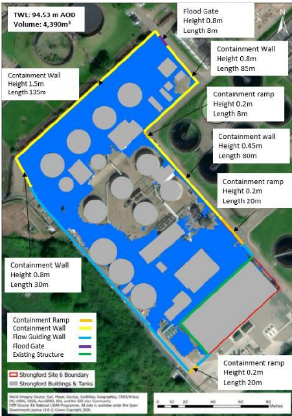
Figure ii – recommended solution for the digester area
