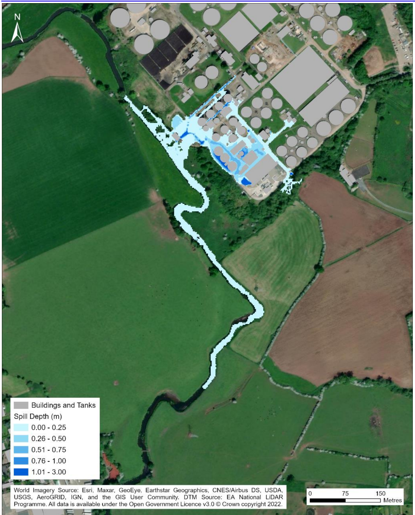
Figure 2.3 Uncontrolled spill of Strongford STW (Depth Profile)
