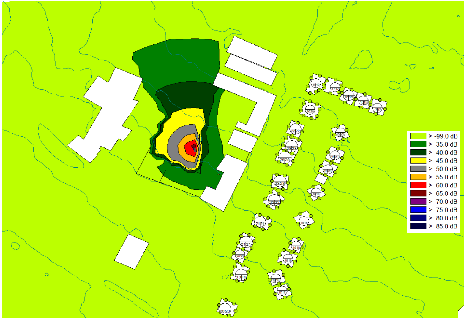
Figure 5.3 - Assessment of typical nighttime noise sources associated with the tipping activities as per BS4142:2014
