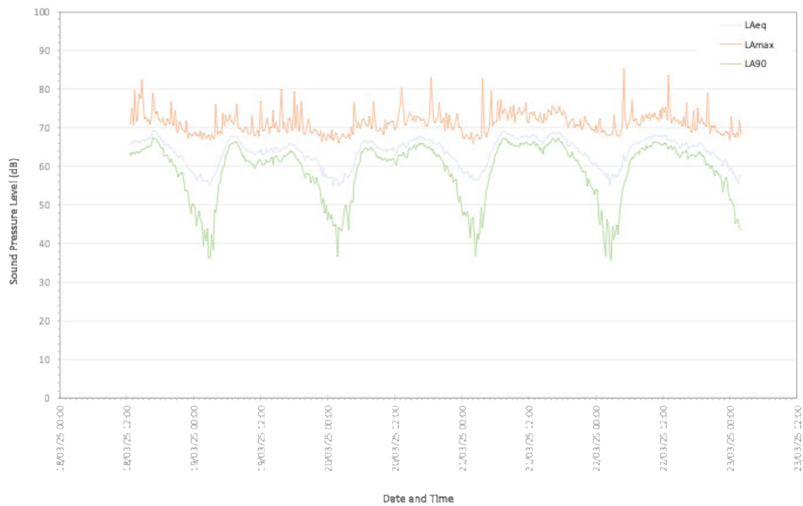
Figure C1: Background Noise Survey Results, Drayton Park
