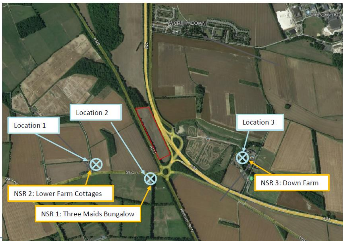
Figure 4.1 – plan showing locations of sound level measurement positions used to monitor sound from the site (Figure 5-2 of the Noise Impact Assessment, SLR Consulting 1 )
