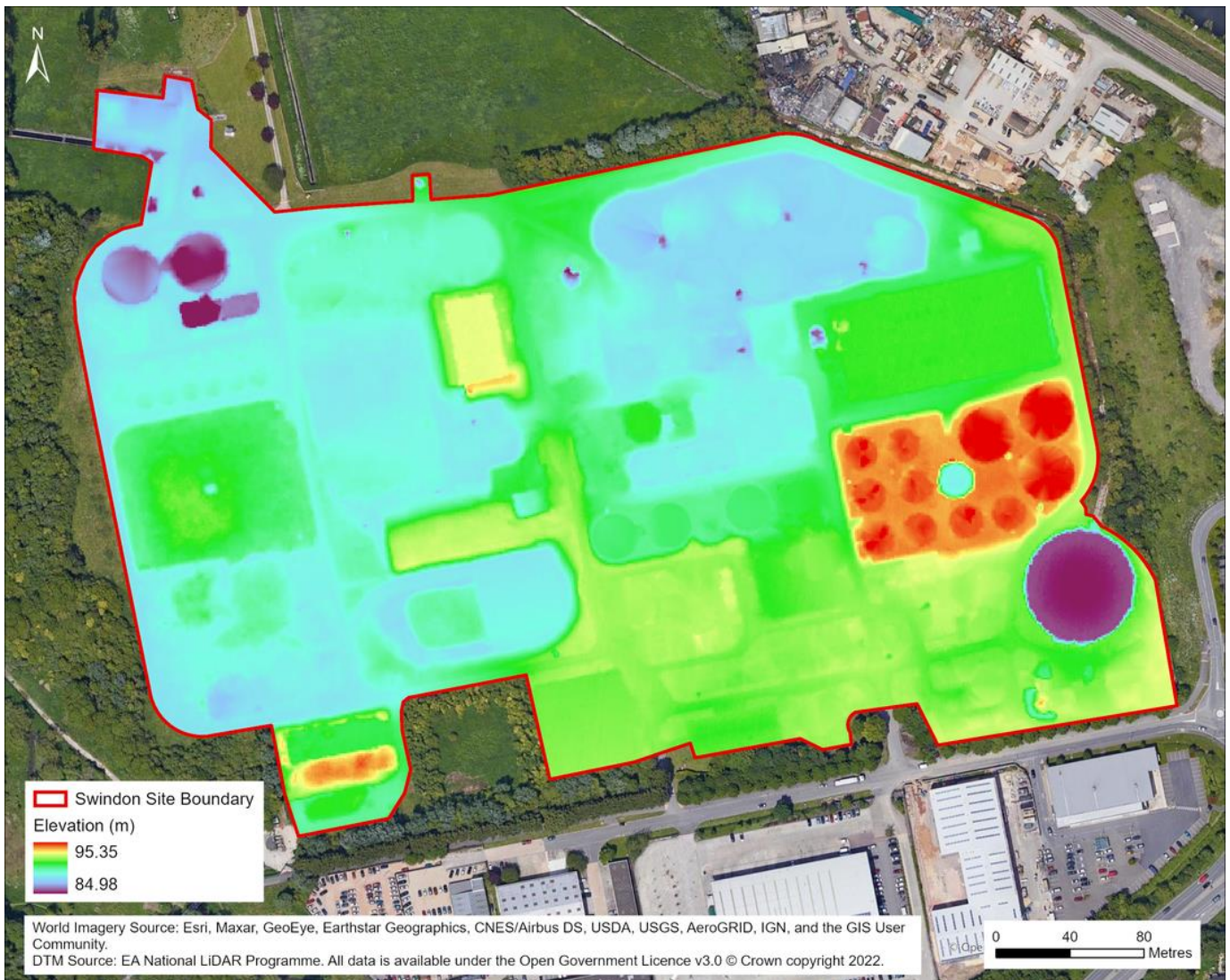
Figure 5: Digital Terrain Model of Swindon STW
