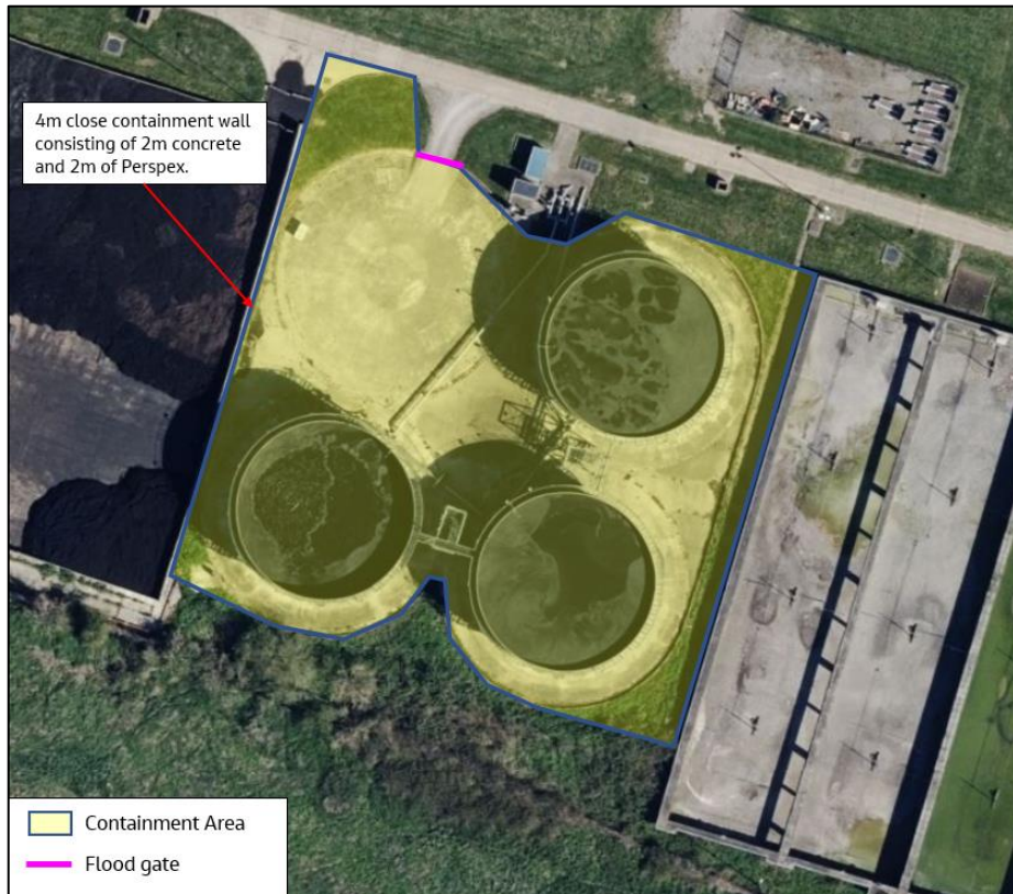
Figure 1-3 – Secondary Digesters Area – Containment layout
