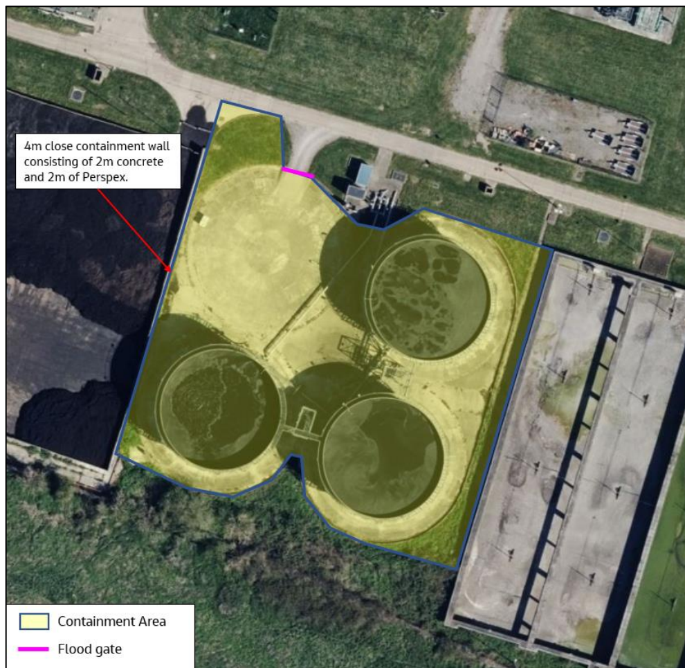
Figure 4-11 – Secondary Digesters Area – Containment Solution
