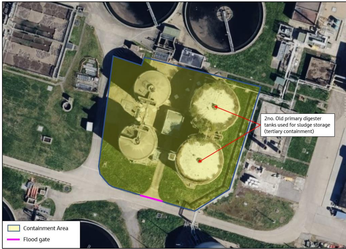
Figure 1-1 – Primary Digesters (south-west) Area – Containment layout
