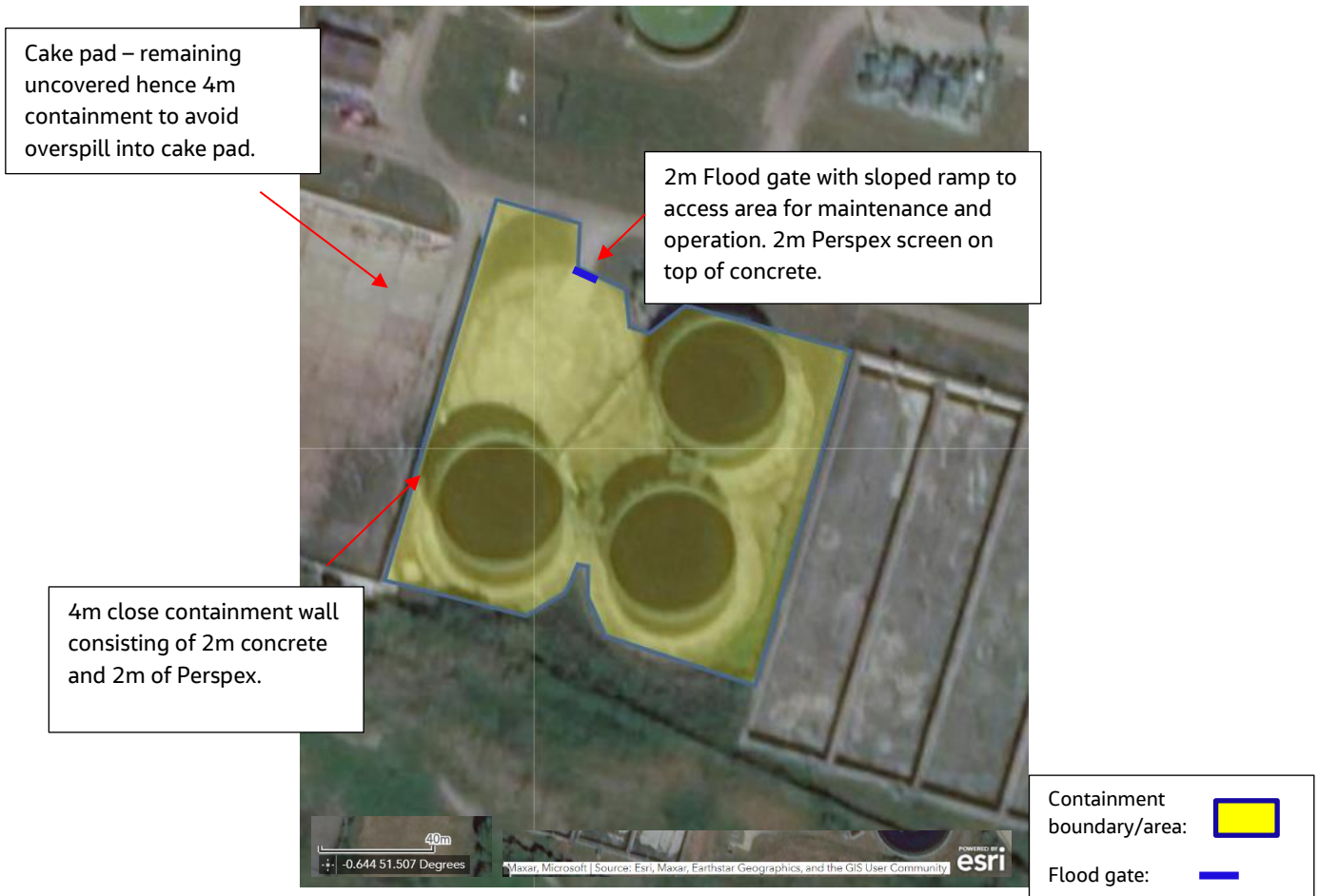
Figure 4.4 Secondary digester area - containment option
