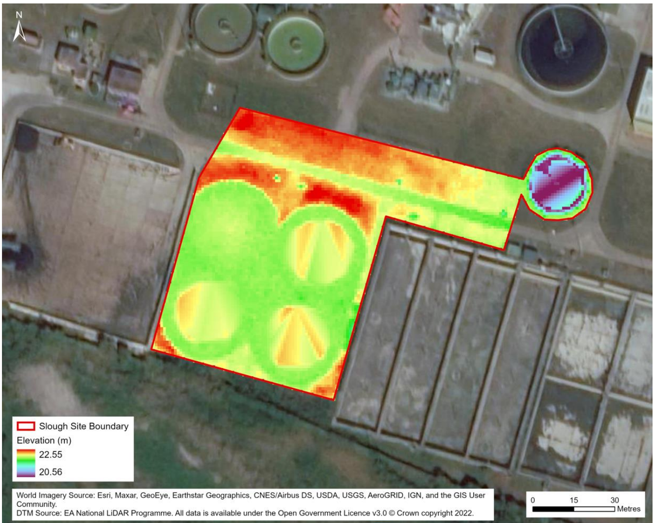
Figure 3.6 Digital Terrain Model of Slough Sewage Treatment Works
