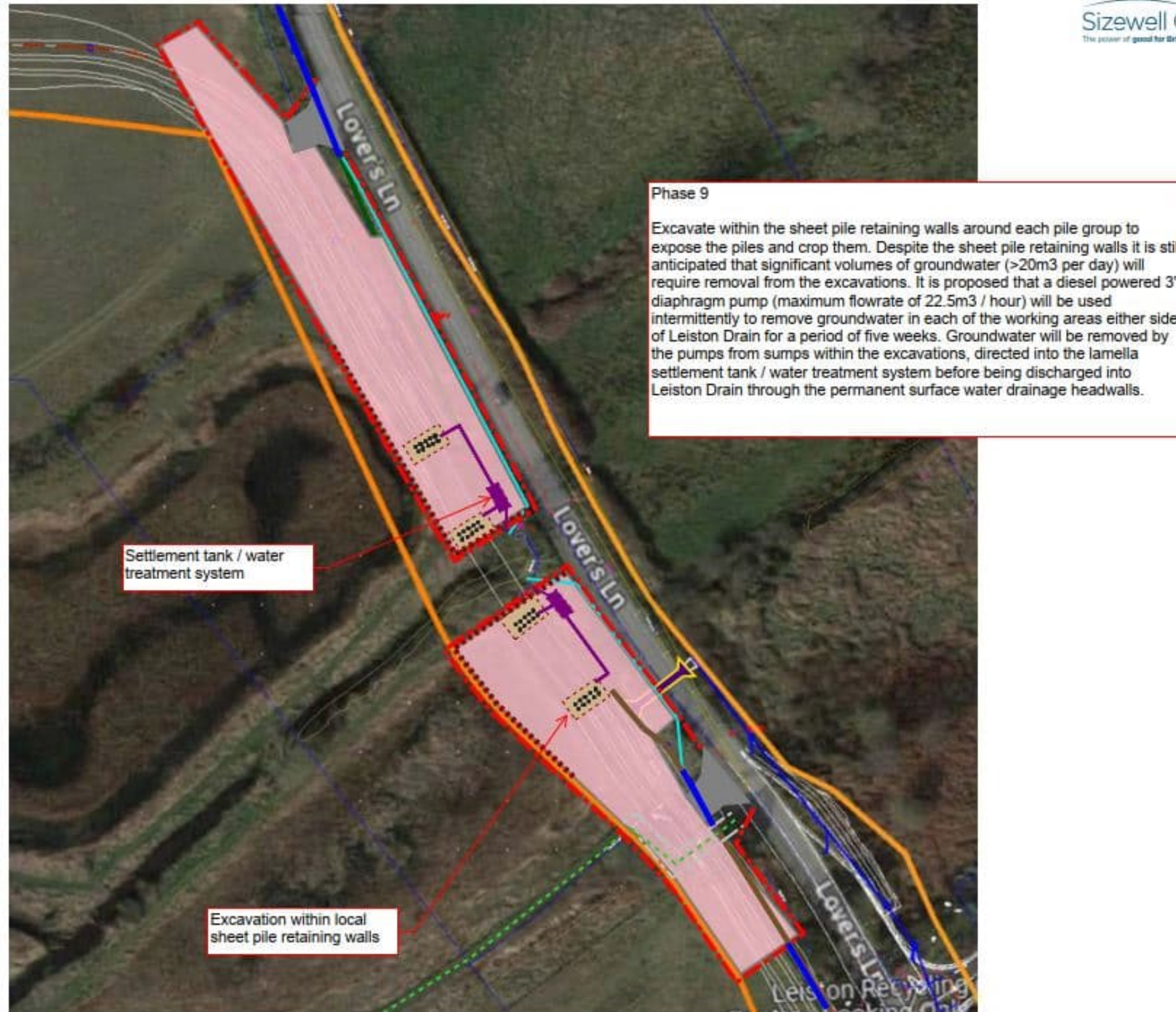
Figure 1 – Location of settlement tanks
