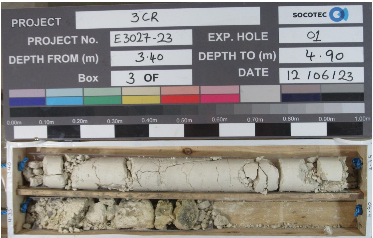
BH-01 Core 3.40 to 4.90m
