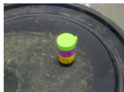
Wire has been detached and lid replaced to ensure insulation of terminals. If a lid is not available apply tape to isolate
