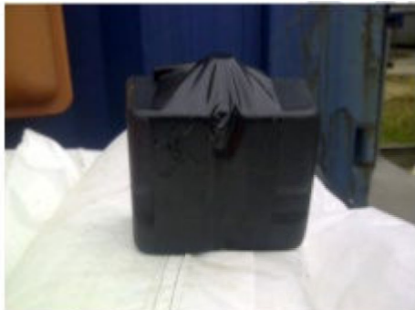
Lithium battery with terminals insulated.
