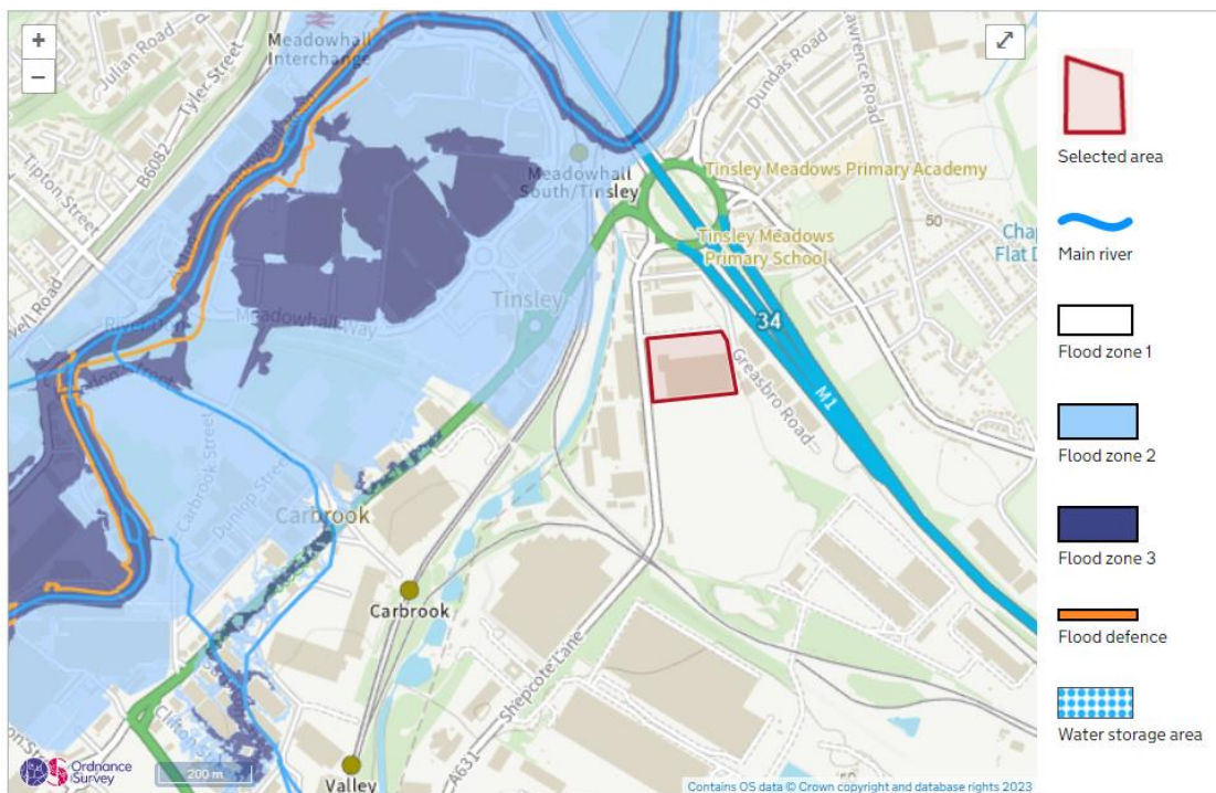
Image 3.1: Installation boundary and flood zone assessment
