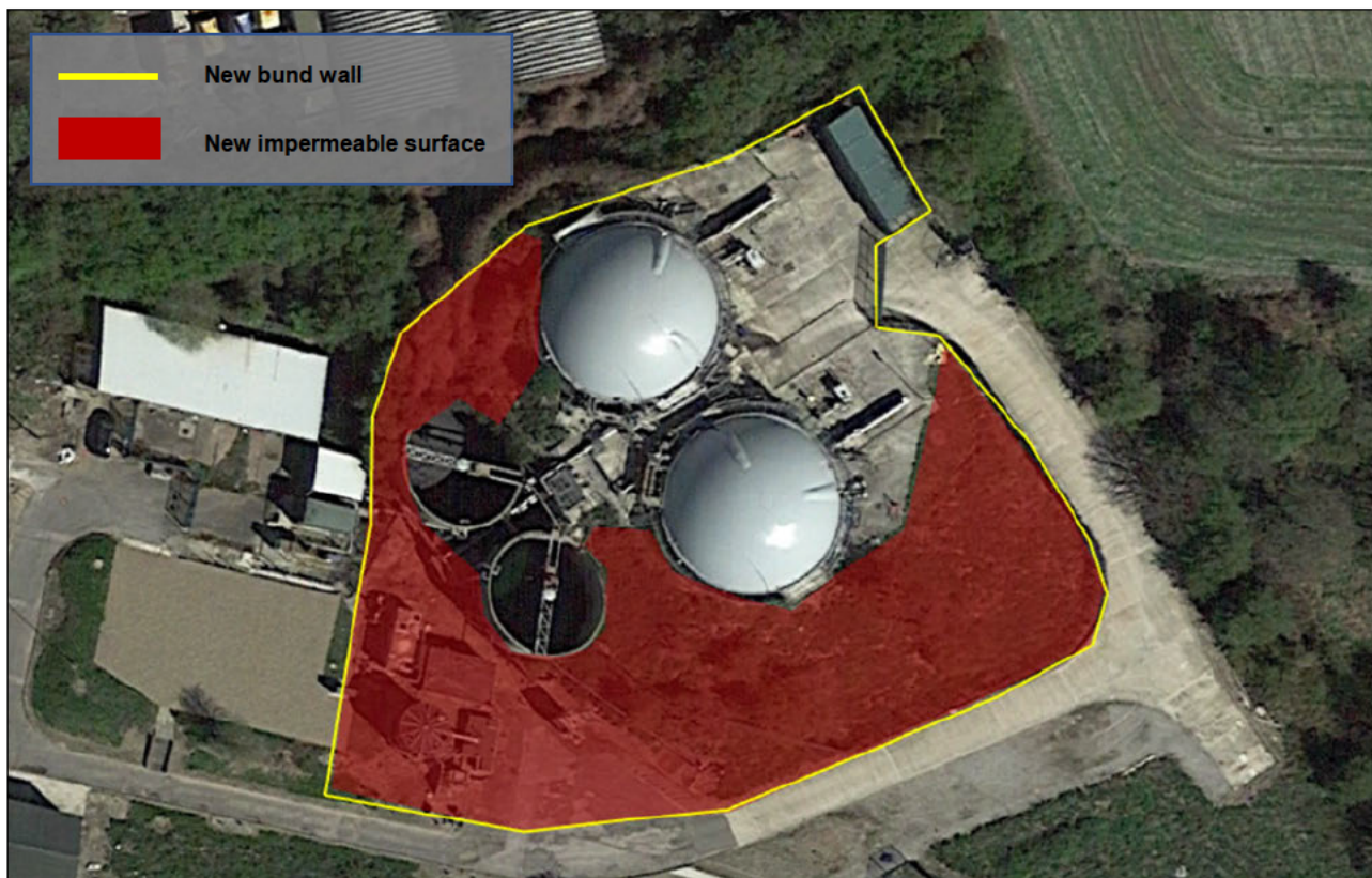
Figure 33. Mitigation - multi-tank area 3
