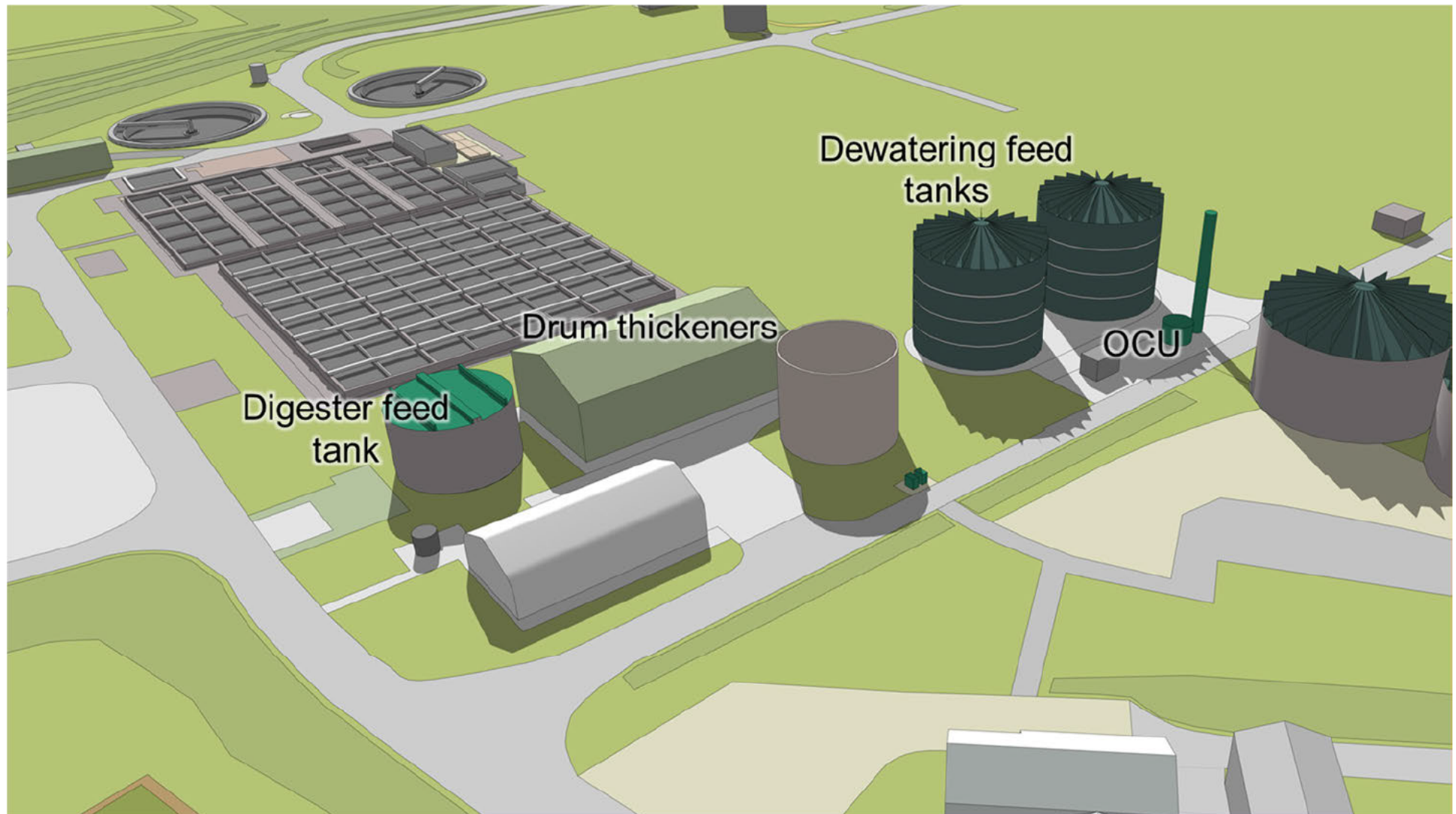
Figure F Site view showing raw sludge thickening area
