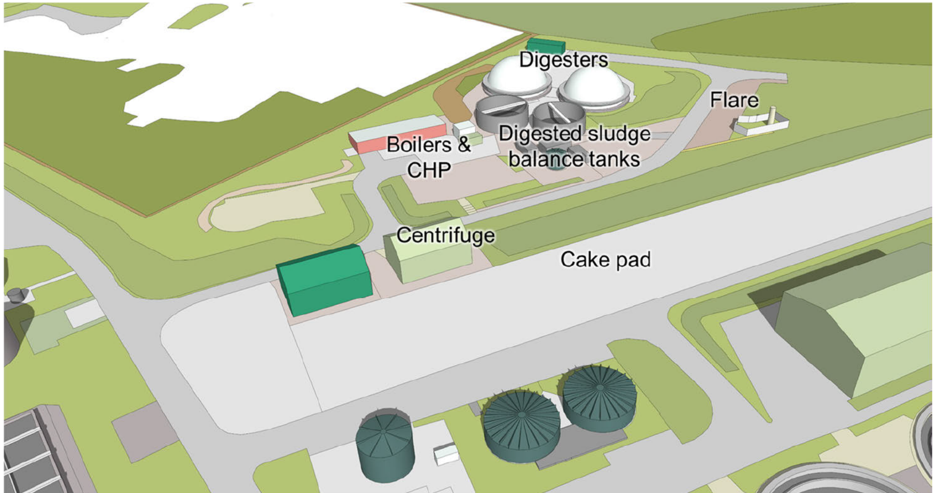
Figure I Site view showing digesters and areas of biogas storage and use
