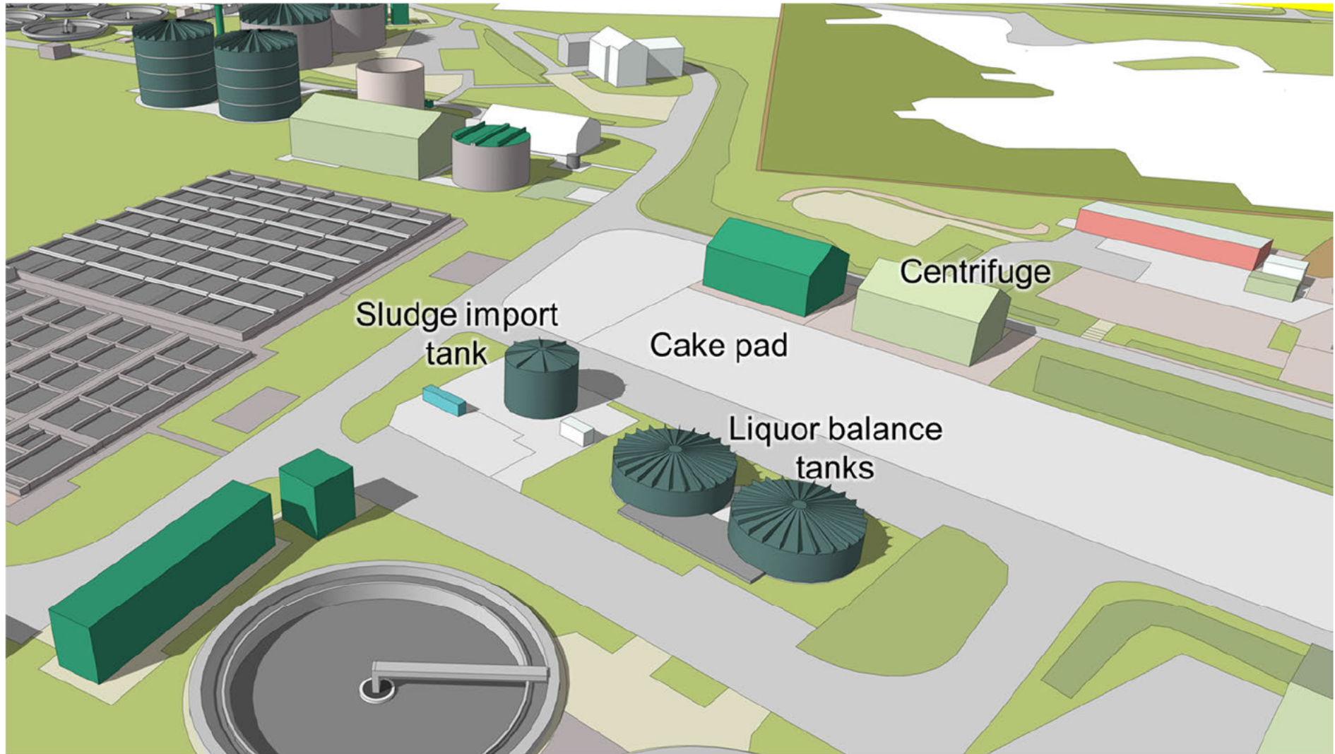
Figure K Site view showing sludge intake area and digested sludge dewatering area
