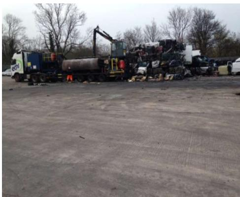
All the vehicles after depollution are baled and sent to a shredder operator as a scrap metal for recycling. The activity is taking place in the scrap car baling area.
