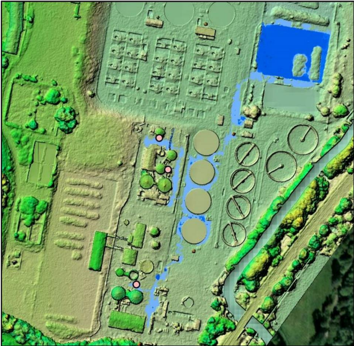
Figure 20. Model showing unmitigated result of spills from existing tanks at Old Whittington using the CIRIA C736 rule.
