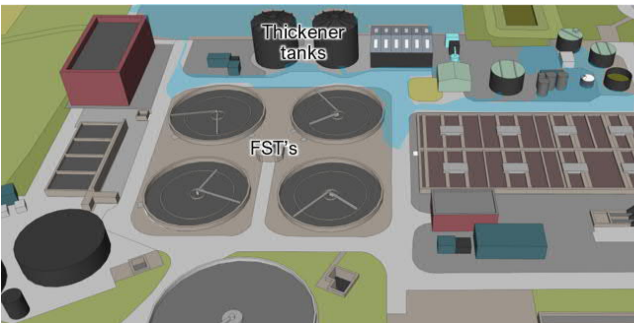
Figure 21. Potential pooling around the thicker tanks and FST's.
