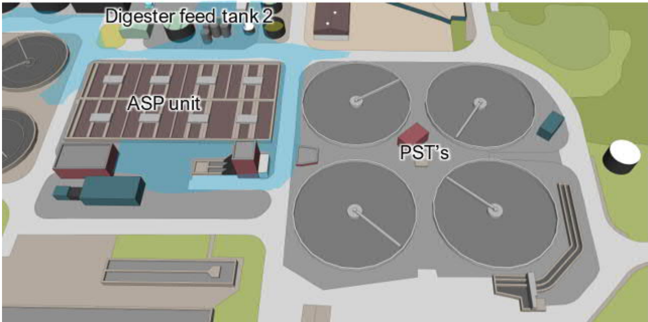
Figure 22. Potential pooling around ASP's and PSTs, plus surge potential from digester feed tank no 2.
