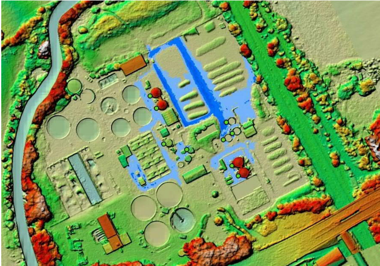
Figure 18. Model showing unmitigated result of spills from existing tanks at Woodhouse Mill
