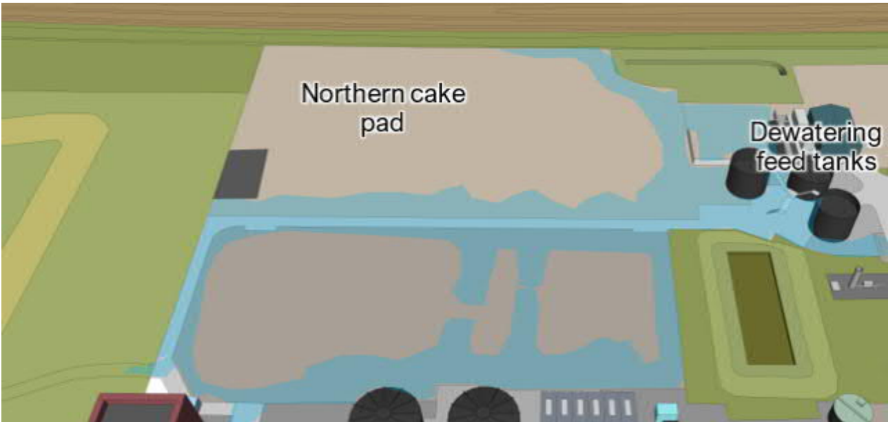
Figure 20. Pooling potential within the northern cake pad and around the dewatering tanks.
