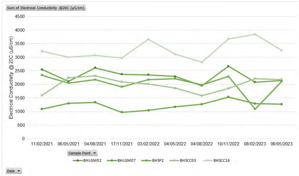
Figure 4-4 Conductivity chemograph of baseline groundwater quality
