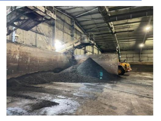
Digested sludge cake falls from conveyors into the Cake Barn which is odour abated via an OCU.
