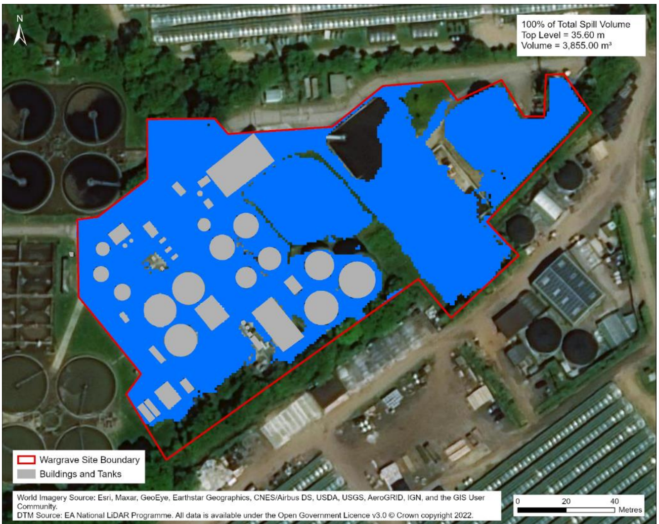
Figure 3-4 - Containment spill model
