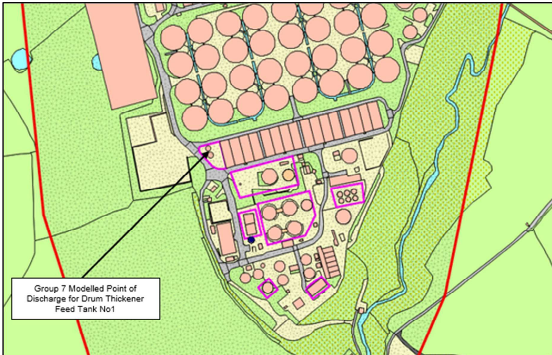
Figure 19: Blackburn STC Modelled Point of Discharge for Drum Thickener Feed Tank No 1 Burst
