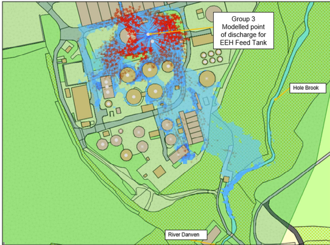
Figure 12: Blackburn STC Predicted Flow Paths following EEH Feed Tank Burst
