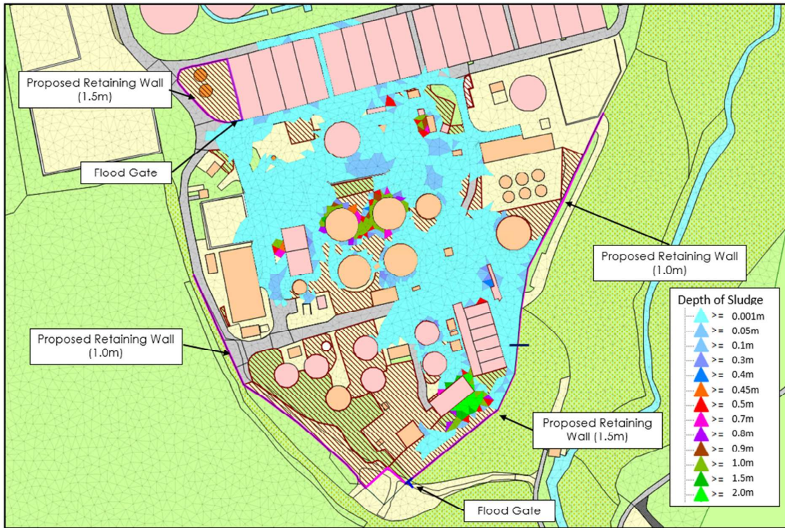
Figure 31: Proposed mitigation and settled sludge depth for Group 3- EEH Feed Tank
