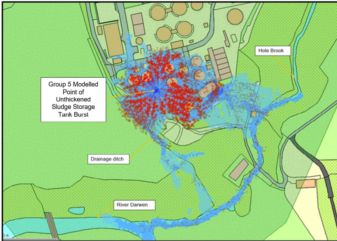
Figure 16: Blackburn STC Predicted Flow Paths following Unthickened Sludge Storage Tank Burst
