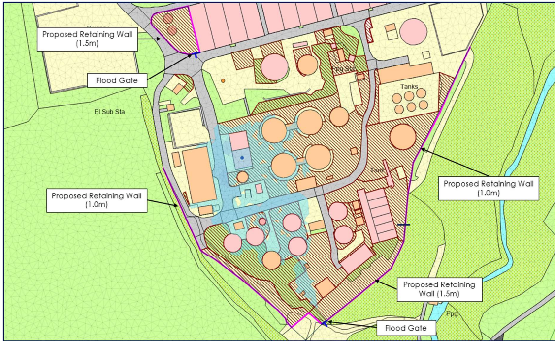
Figure 23: Proposed mitigation and flood extent for Group 2- Post Digestion Tank
