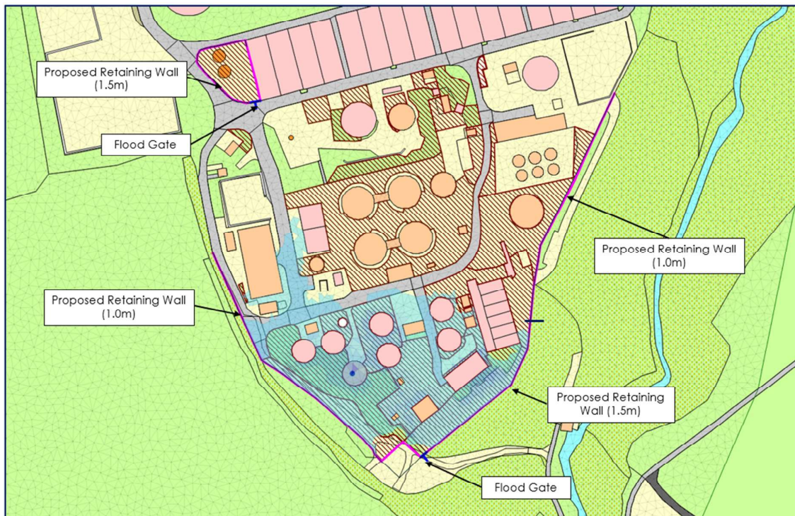
Figure 25: Proposed mitigation and flood extent for Group 4 - High Rate Enzymic Hydrolysis (EEH) Tanks
