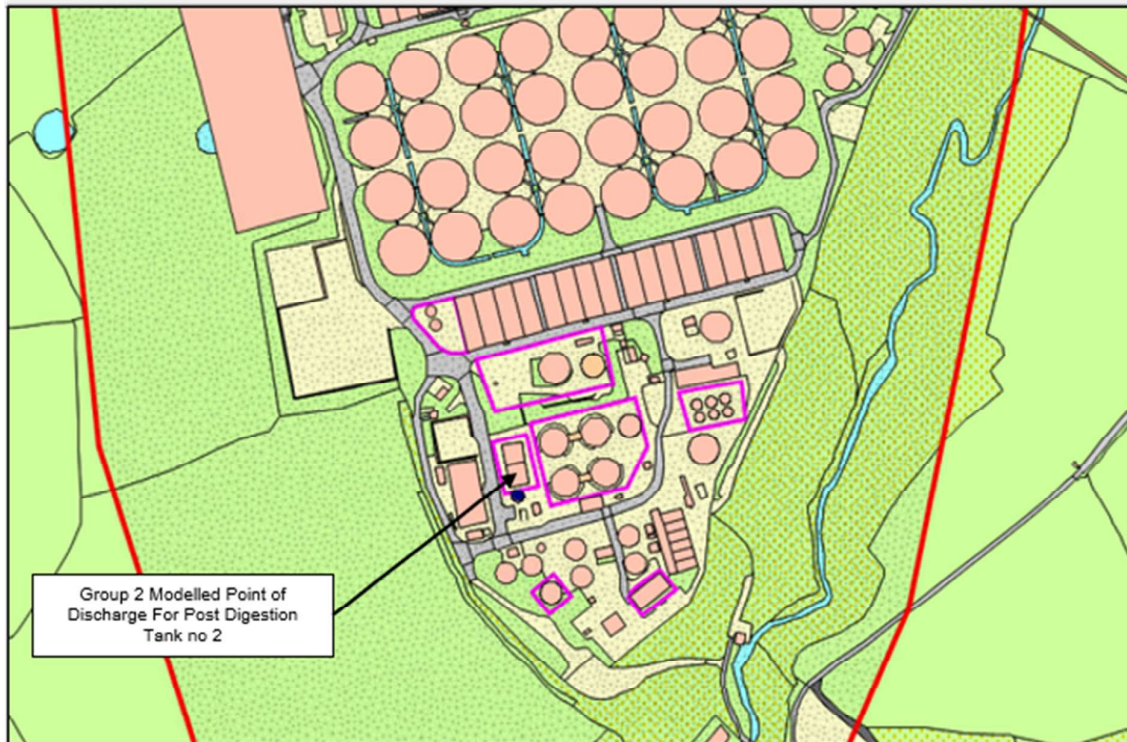
Figure 9: Blackburn STC Modelled Point of Discharge for Post Digestion Tank no 2 Burst
