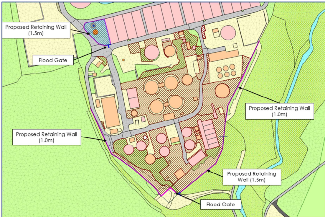
Figure 27: Proposed mitigation and flood extent for Group 6 – Centrate and Filtrate Tank
