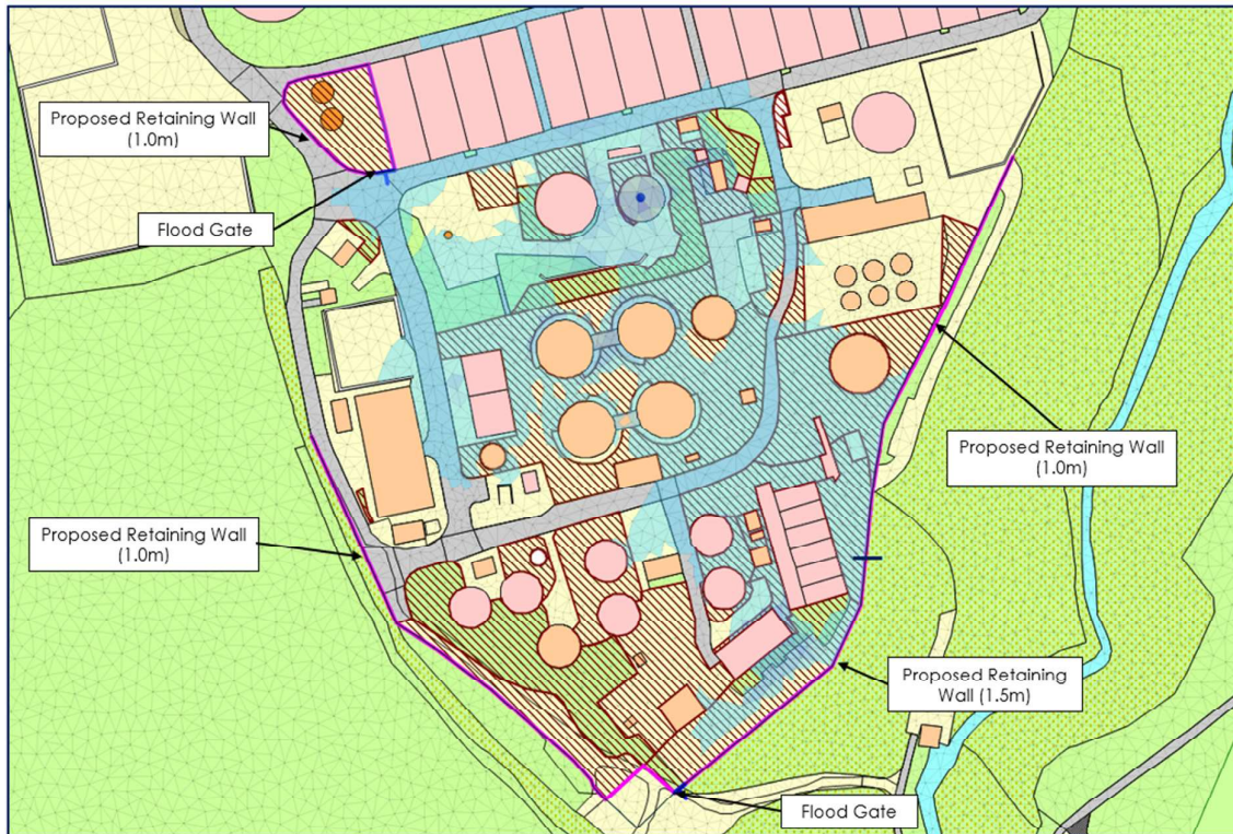
Figure 23: Proposed mitigation and flood extent for Group 2- Post Digestion Tank
