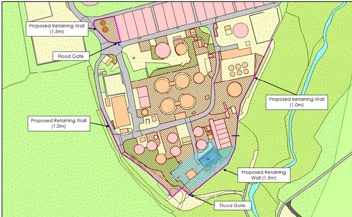
Figure 27: Proposed mitigation and flood extent for Group 6 – Centrate and Filtrate Tank
