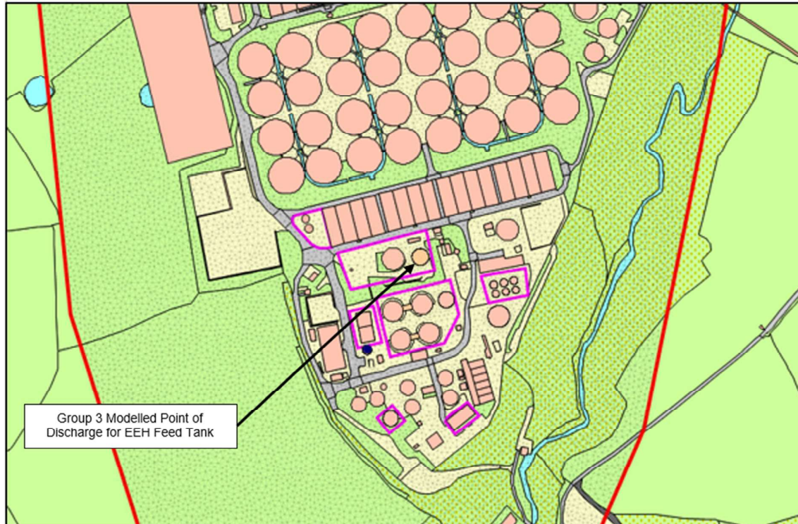
Figure 11: Blackburn STC Modelled Point of Discharge for EEH Feed Tank Burst
