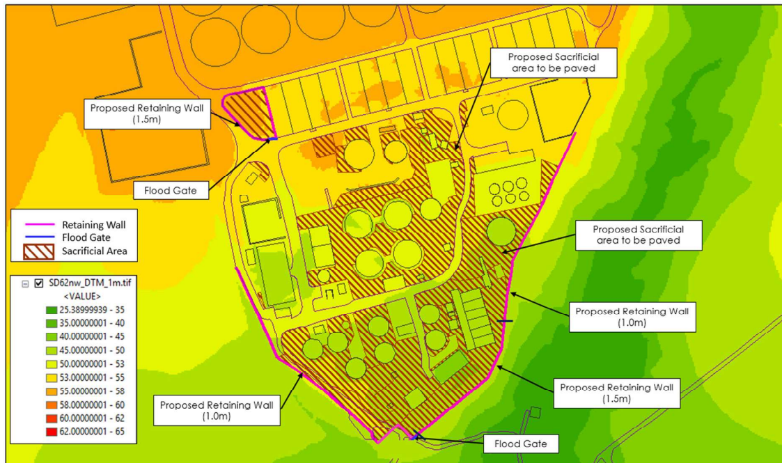
Figure 31: Ground Levels and Proposed Mitigation Measures
