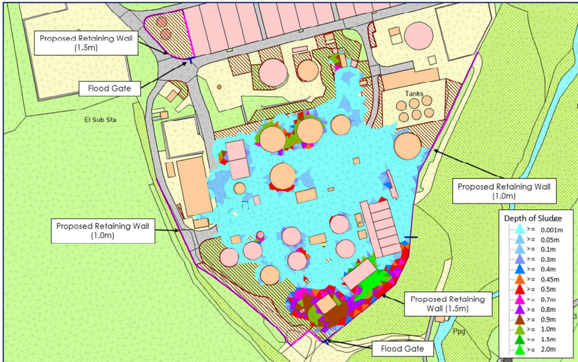
Figure 29: Proposed mitigation and settled sludge depth for Group 1- Digester
