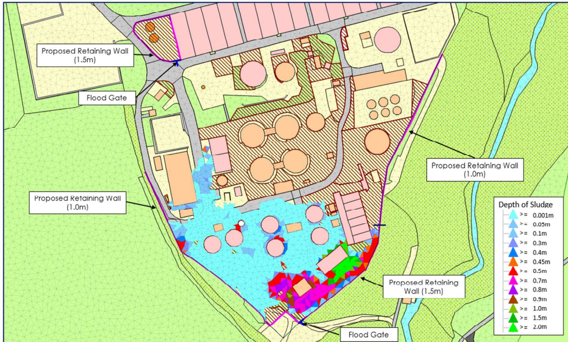
Figure 33: Proposed mitigation and settled sludge depth for Group 5 – Unthickened Sludge Storage Tank
