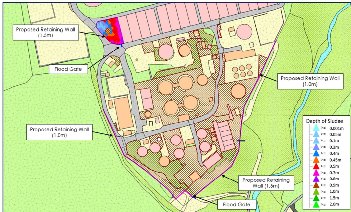
Figure 35: Proposed mitigation and settled sludge depth for Group 7 – Drum Thickener Feed Tank
