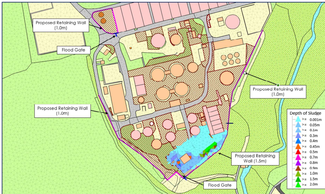
Figure 33: Proposed mitigation and settled sludge depth for Group 5 – Unthickened Sludge Storage Tank
