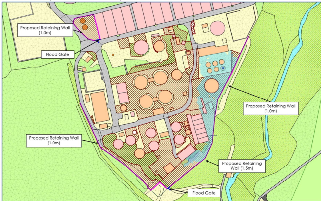
Figure 25: Proposed mitigation and flood extent for Group 4 - High Rate Enzymic Hydrolysis (EEH) Tanks
