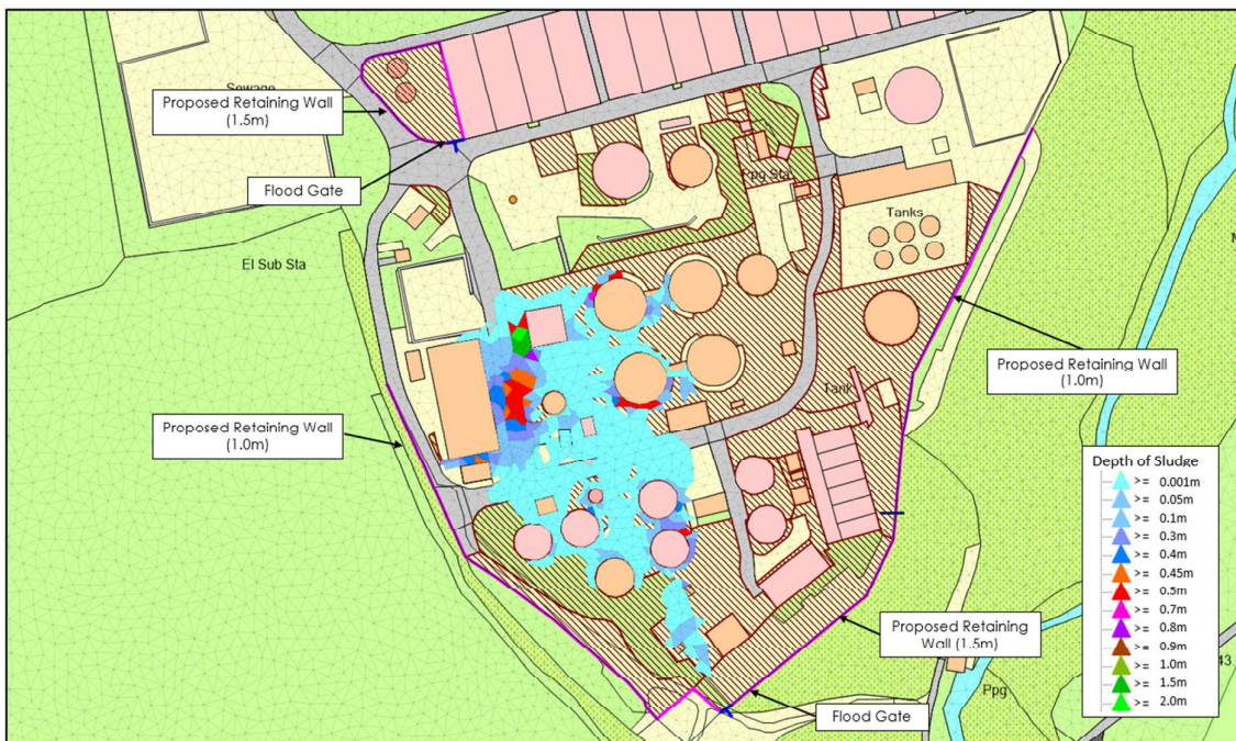
Figure 29: Proposed mitigation and settled sludge depth for Group 1- Digester
