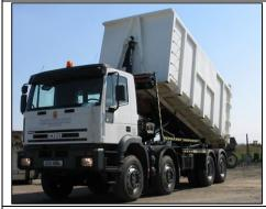
To transfer cake to treatment centre the sealed container is removed by hook lorry and transported to the centre, sealed and unopened.
