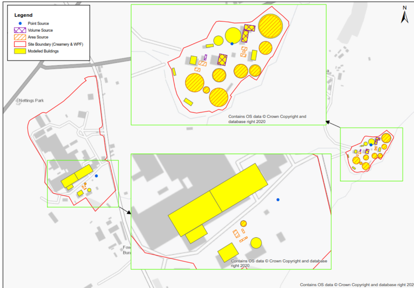
Figure 7 Modelled buildings included to represent building downwash effects
