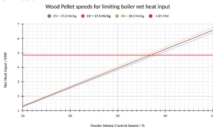
The boiler trials concluded that, in order to ensure that the net heat input is <5 MWth, the feeder speed must be below 37% equivalent to 4.85 MWth.
