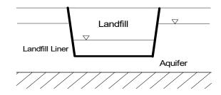
The landfill is constructed in a clay pit, underlain by a confined aquifer. Water and contaminant fluxes occur across the bottom of the landfill only.
