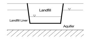
The landfill is constructed in a clay pit, underlain by a confined aquifer. Water and contaminant fluxes occur across the bottom of the landfill only.
