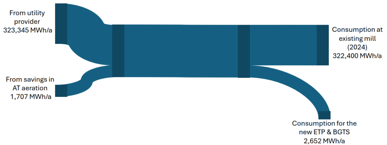
Figure 3-1 - Sankey Energy Balance Diagram Electricity
