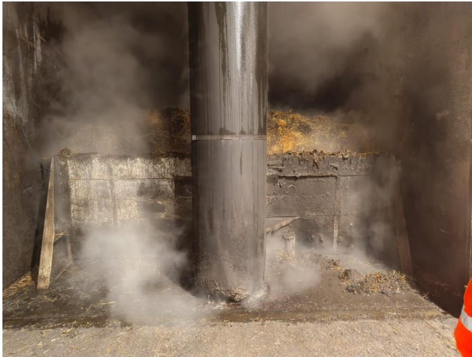
Figure 2 - aerated material biodrying during trial
