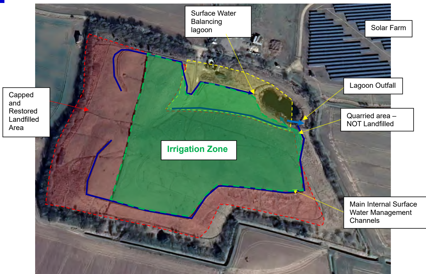
Figure 2 Irrigation Zone within Capped and Restored Area Captured by Surface Water Drainage Zone
