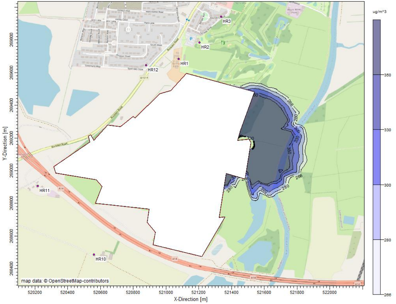
Figure B-3 15-minute Mean (99.9%ile) Sulphur Dioxide Process Contribution (Sc2)
