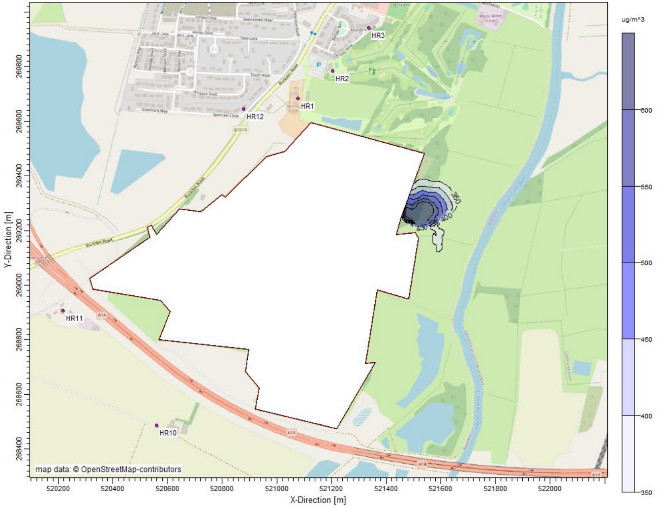
Figure B-6 1-hour Mean (99.73%ile) Sulphur Dioxide Process Contribution (Sc2)
