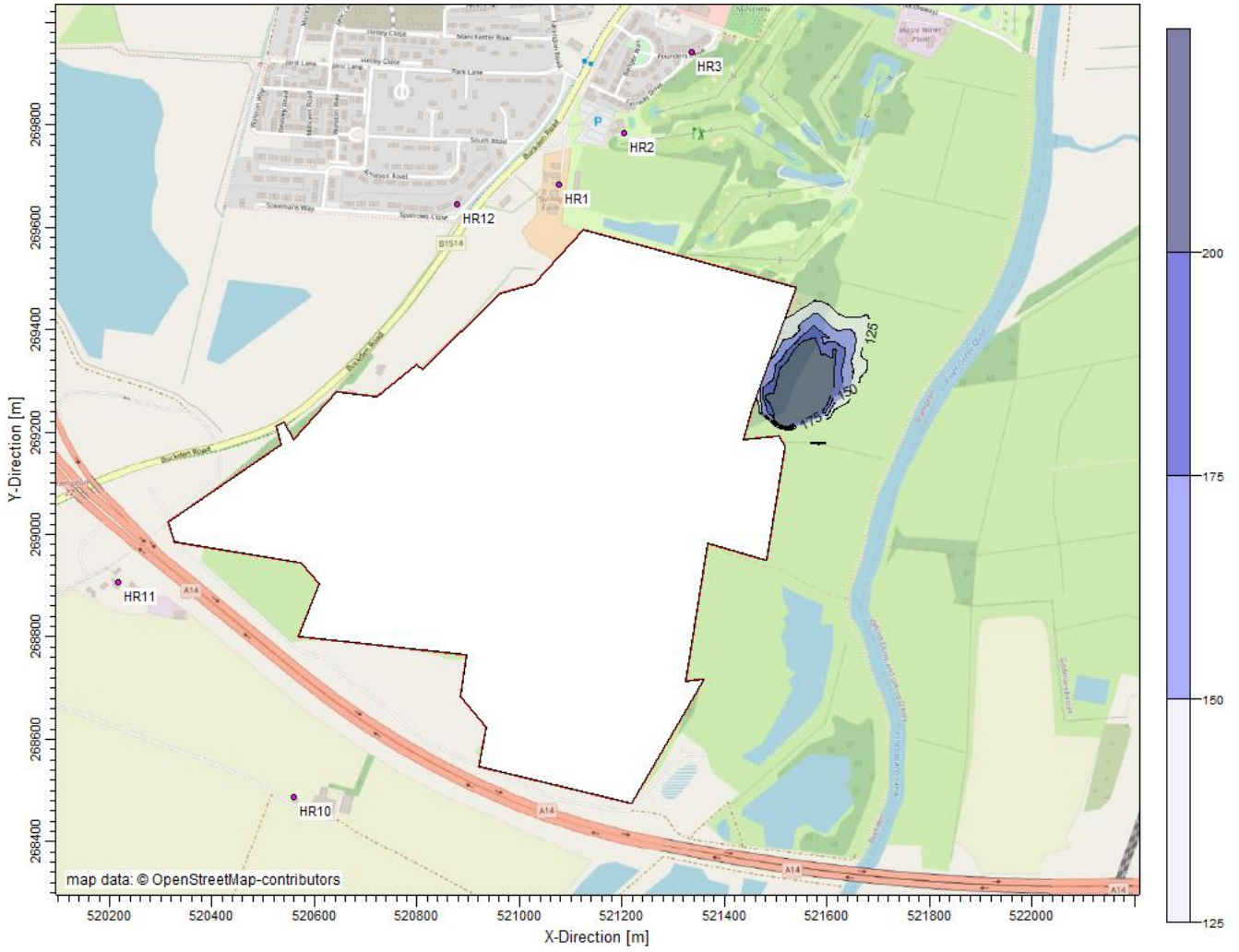
Figure B-9 24-hour Mean (99.18%ile) Sulphur Dioxide Process Contribution (Sc2)
