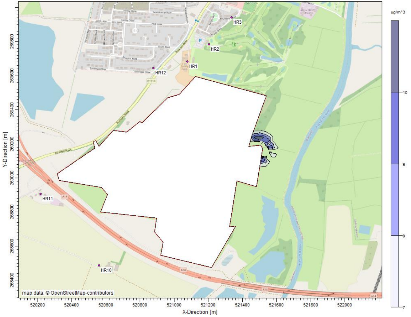
Figure B-13 30-minute Mean Hydrogen Sulphide Process Contribution (Sc2)
