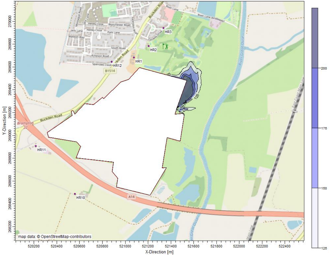
Figure B-8 24-hour Mean (99.18%ile) Sulphur Dioxide Process Contribution (Sc1)
