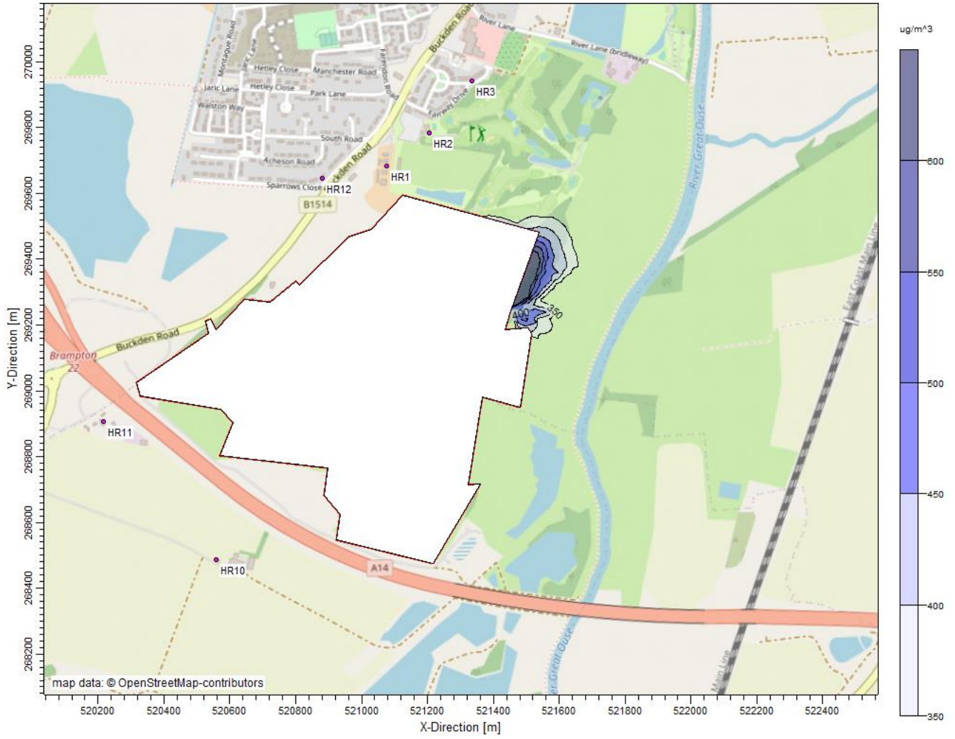
Figure B-5 1-hour Mean (99.73%ile) Sulphur Dioxide Process Contribution (Sc1)
