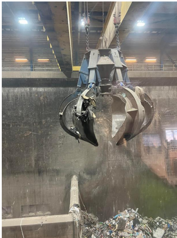
Graphic 3.3: A typical waste bunker crane
