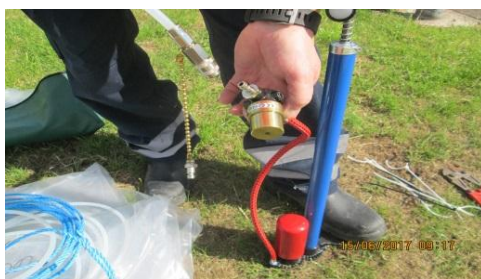
Connect white hose to pump insert bladder in drain and pump up Pump and hose connection
