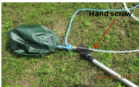
Pull back knurled collar to ensure air release valve on chain is undone
