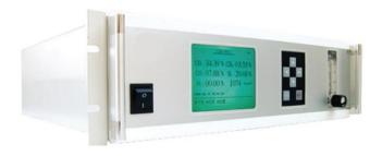
Professional online gas analysis systems for continuous monitoring of pyrolysis and gasification processes.
