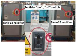
Switch "off" the anodising tank rectifier from back side of the tank .
