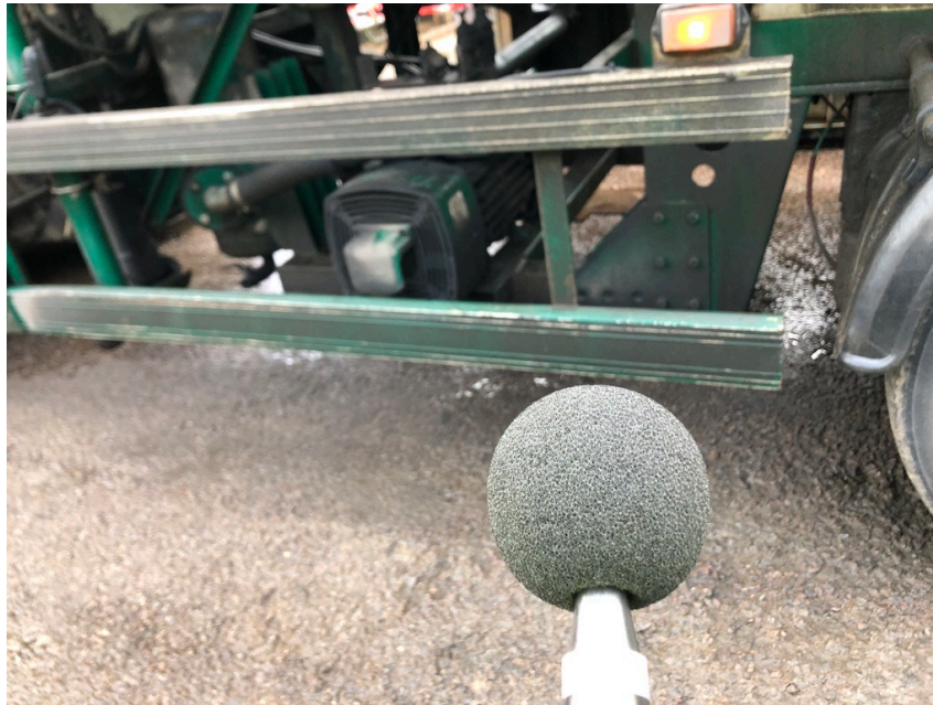
Figure 5: The vacuum pump on the truck and the location of the sound level meter microphone
