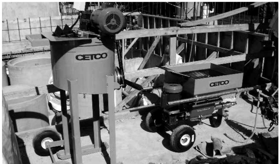
Figure 2: CETCO pump and mixer with electric 1HP motor
