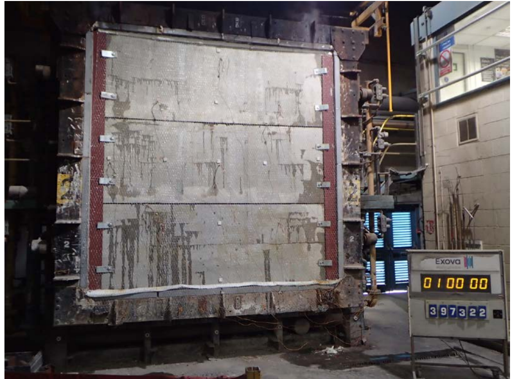
The unexposed face of the test specimen after 60 minutes of testing
