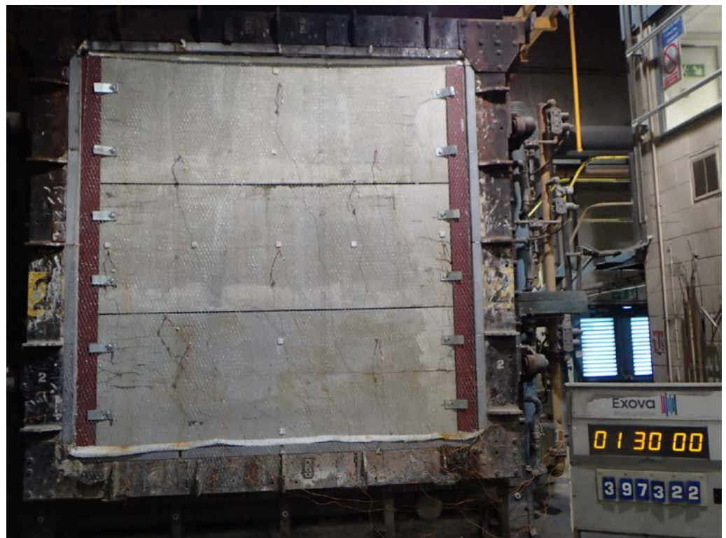
The unexposed face of the test specimen after 90 minutes of testing
