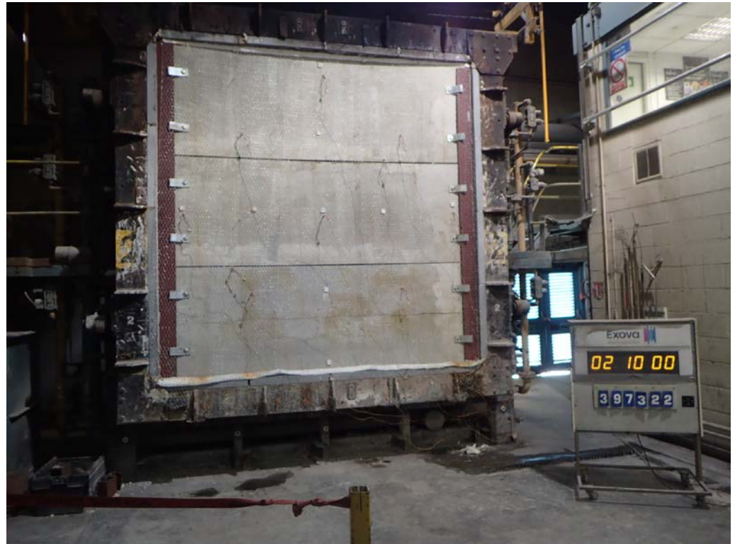
The unexposed face of the test specimen after 130 minutes of testing
