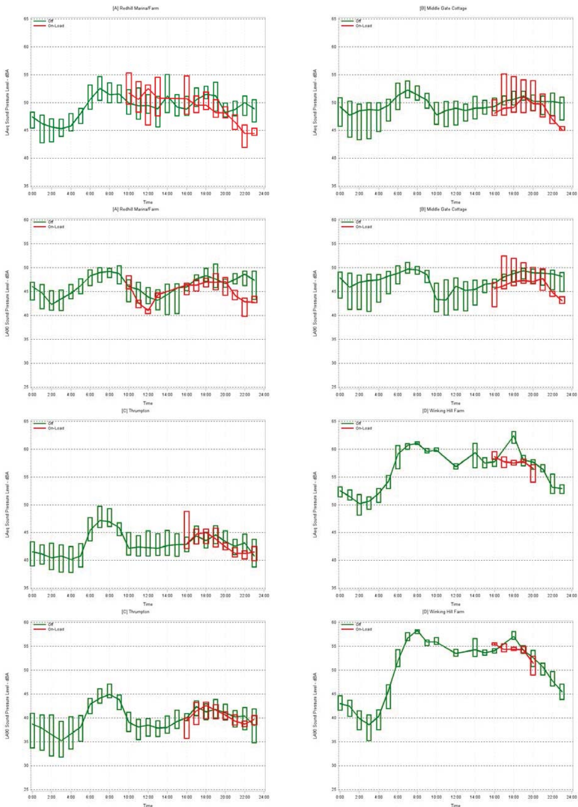
Figure 16: Diurnal Variation of L_{Aeq} and L_{A90} at Receptors [A] to [D] (Power Station off-load or on-load)
