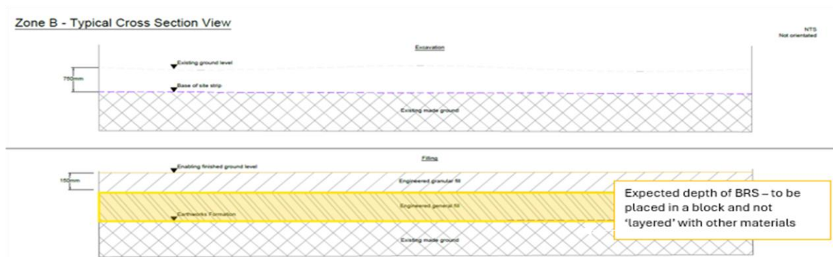
Figure 2 - Indicative cross section and layering of BRS in Zone B
