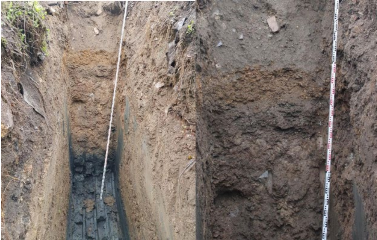
Left: Natural alluvium at the base of the trial pit. Right: layers of Made Ground within the mound including yellow brown sandy gravel and brown sand with grey sandy clay.
