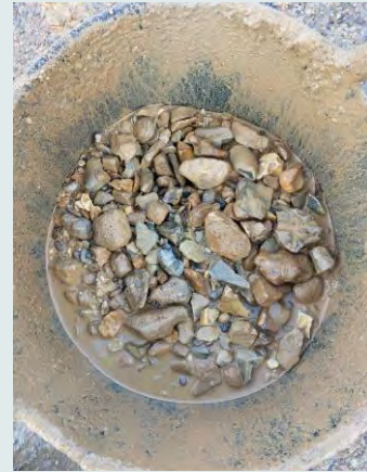
View of Granular Segment of the River Terrace Deposits from BH3
