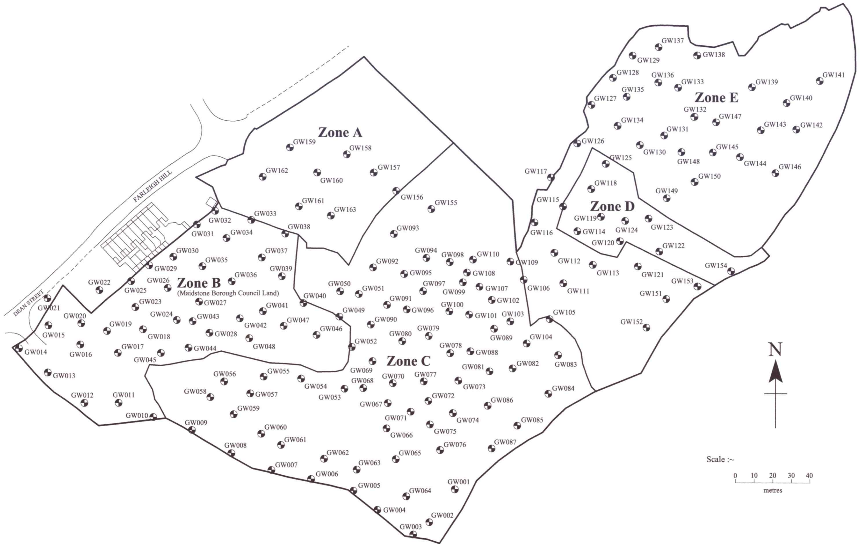
Fig. 6. TOVIL QUARRY - 2005/6 Investigation - Gas spike locations
