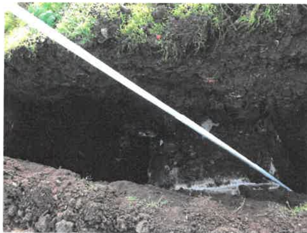
Concrete block (old floor slab) noted at 1.40mbgl.
