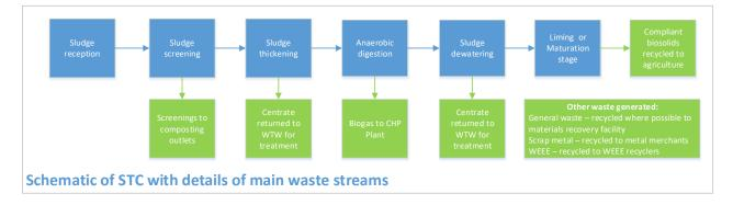
A schematic of the main waste streams from the STC is shown below.
